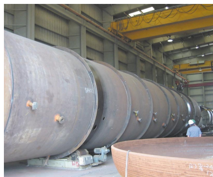
One of two huge Deaerator Towers destined for Angola, in NATCO's New Iberia fabrication shop
