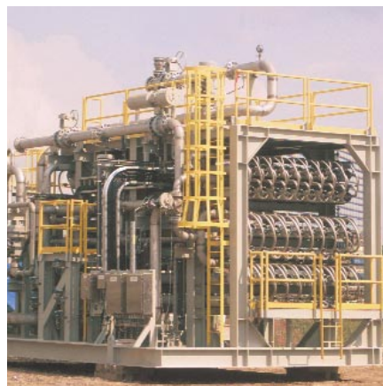
One of seven membrane modules capable of producing 350,000 bpd low sulfate seawater for Kizomba A field at NATCO's New Iberia facility
